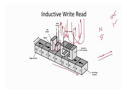
Now the read write head will look something like that. So, this is basically you can see that we are having a mechanism like that some iron or coil iron substrate inductive write element. So, here we are going to have a coil, we are going to put a coil. So, it is very much similar to I can tell you some sort of your DC electrical motors or electrical generators.
